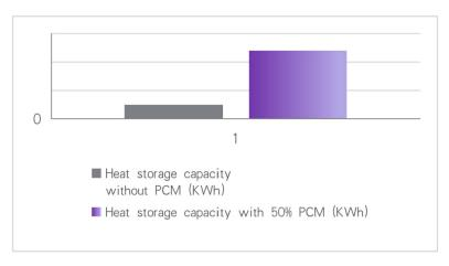
Lab result: heat storage capacity increase from 2kwh to 12.2kwh
